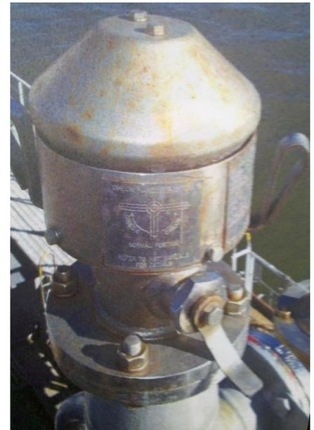
After this specific casualty, the high velocity vent valve of the tank being filled was found stuck closed and inoperable using the manual test lever. A valve for another tank was also found stuck. Scientific testing of the substance between the stuck valve disc and the seating surfaces indicated the presence of oxidized vegetable oil or fat likely from previous cargoes. It appears doubtful that crewmembers exercised the valves prior to their cargo operations as per their operating procedure.
